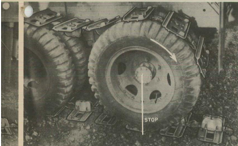
Figure 8. This is what your truck looks like if you've lagged along through the first photos. The truck is stopped right here, so only TWO shoes are left sticking out from under the tire.
