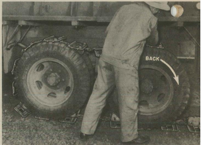
Figure 7. Still inching the truck back. The last shoe over and will go around the other side fast now, like a chisel. He's watching his own shoes, too, staying well away from the track.
