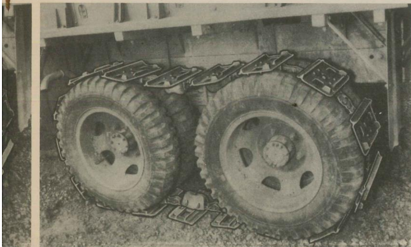
Figure 11. The sway back is gone. The track FEELS snug. It even LOOKS tight. A road test will really tell. Hold your horses till you get tracks on the other rear bogie and on the front duals.
