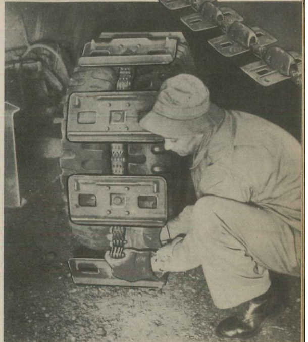
Figure 12 (upper photo) Nothing's special about slipping the track on the front tires. First put on the spare wheel. That's easy . . . just drive the front wheel up on a board. That's to get clearance enough to put on the spare wheel. Stretch the tracks out in front, and hop to it. (Lower photo) The same system used in Figure 5, but with the truck moving FORWARD, brought the track around to here. Now Joe's joining up the last shoe on the ground. Next he'll tighten each shoe (as in Figure 10), till the track's snug.
