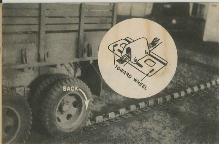
Figure 3. Two bruisers just dragged the track around back of the truck. Place the track so the edge of the shoe with the SHORT CLEATS FACES the tire; the edge with the LONG cleat faces AWAY from the tire.
